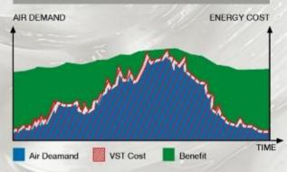
EKO - VST compressors are driven by a frequency converter. Factory air demand is measured continuously and the motor speed is automatically adjusted accordingly. Thus, the compressor produces compressed air by using only as much energy as needed, avoiding unnecessary waste.
