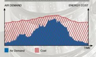
Standard compressors run with load - unload mode between two pressure points. When the pressure reaches the maximum level, the compressor goes unload. During the unload time, the compressor does not produce air; however it consumes about %30 of nominal power
