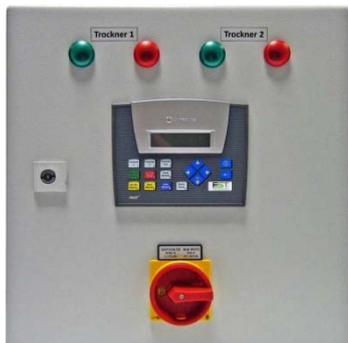
**The DA-CM1-230 switch-over control system** is used to control two redundant compressed air dryers in a compressed air system. These dryers can then be automatically operated alternately. All the dryers provided with a "remote start/stop contact" or a "compressor synchronisation contact" can directly be connected to and controlled by the switch-over control system without the need for modifications.
