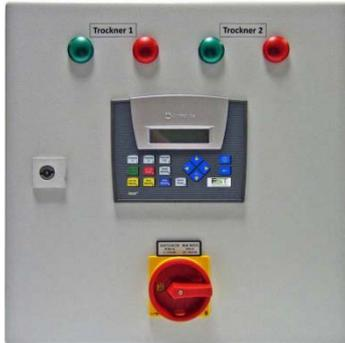
**The DA-CM1-230 switch-over control** system is used to control two redundant compressed air dryers in a compressed air system. These dryer can then be automatically operated alternately. All the dryers provided with a "remote start/stop contact" or a "compressor synchronisation contact" can directly be connected to and controlled by the switch-over control system without the need for modifications.
